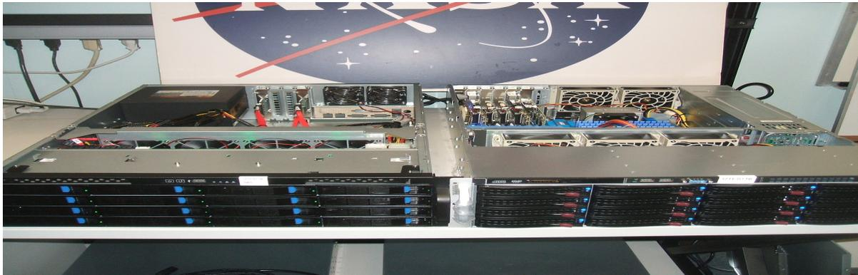
**Figure:** Right case houses Core i7 cores, DDR3 memory, NIC, two “internal” controllers each with eight disks and two “external” controllers; left case houses sixteen SAS-connected disks.
