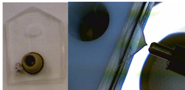
Fig. 5. A tapered electrospray nozzle prototype has been fabricated in glass. Taylor cone formation is shown (right).
